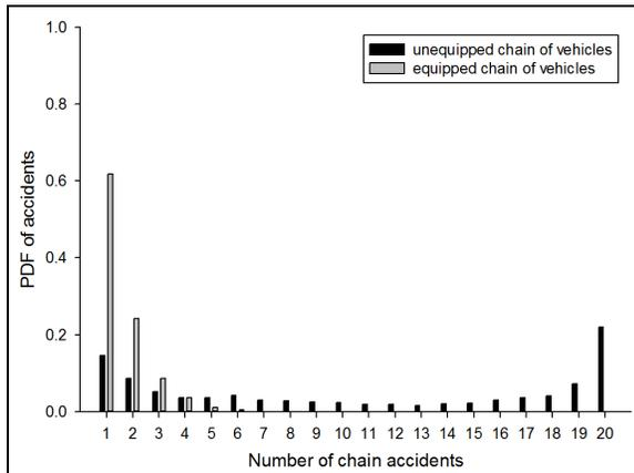
Figure 8. The probability density function of number of vehicles involved in an accident
