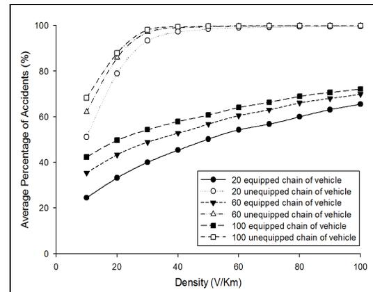
Figure 6. The impact of inter-vehicle communication on average percentage of accidents
