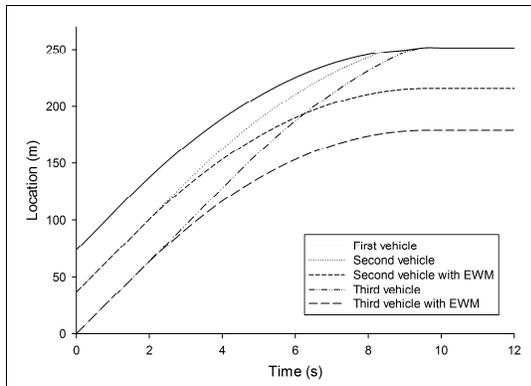
Figure 1. Impact of inter-vehicle communications on collision avoidance
