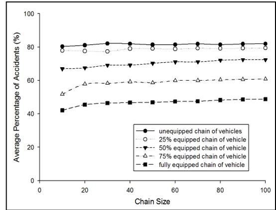
Figure 4. Impact of penetration rate on average percentage of accident for different chain size
