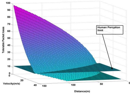
Figure 1. The number of tolerable messages losses with respect to the host vehicle velocity and relative distance to the leading vehicle  $\lambda = 0.1$ .
