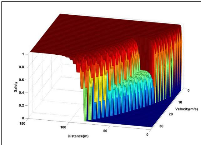
Figure 7. Safety of VH based on its velocity and its relative distance to  $V_L$ .
